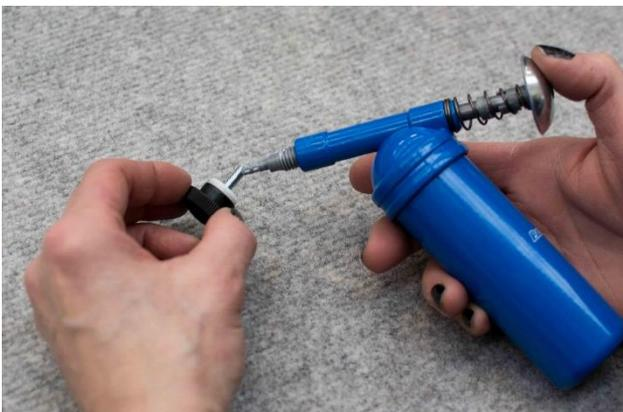
Periodically apply a small amount of anti-seize grease to each thumb screw's thread.
