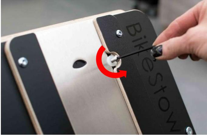
**Carefully** remove the placeholder bolt.
