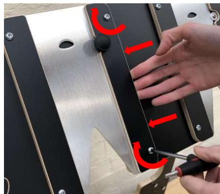
2. While firmly pushing the slider-guide inwards, re-tighten the two bolts.
